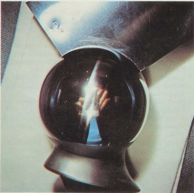
Figs. 15 & 16. Made of Vitallium, the femoral head of this prosthesis has been buffed into a smooth high brilliance, giving the illusion of being a perfect sphere. Actually, the head is not spherical at all, because of previous practical limitations on the
